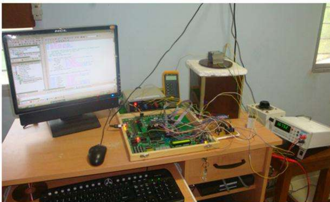
Fig.6. Photograph of the FPGA based temperature measurement & control system
