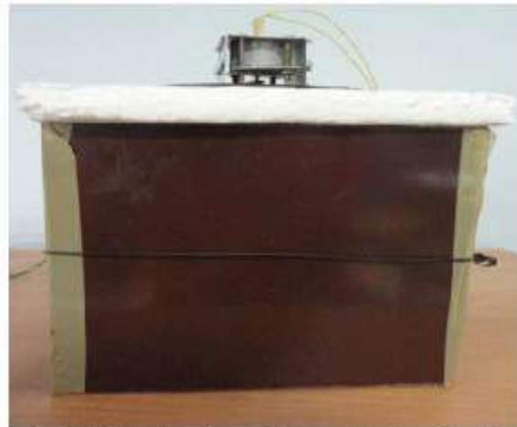
Fig.2. Waterbath with motorized stirrer
